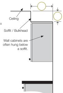
**WARNING:** Soffits typically contain electrical and plumbing elements that can't be relocated. Consult a professional on your remodel.
